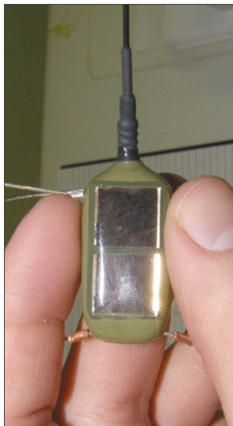
This tiny GPS transmitter has built-in motion and heat sensors and can recharge using solar energy. — Lauren Meads photo
